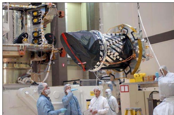
At Lockheed Martin Space Systems in Denver, workers hoist the HiRISE telescopic camera for installation onto the Mars Reconnaissance Orbiter spacecraft, Dec. 11, 2004. HiRISE was built by Ball Aerospace and Technology Corp., Boulder, for the University of Arizona, Tucson. Credit: NASA/JPL/Ball Aerospace
