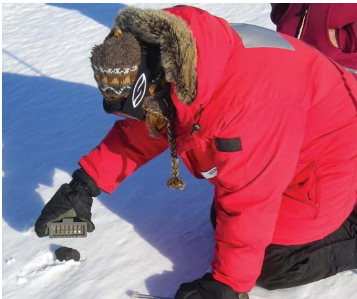
Lane holds a counter near a meteorite, being sure not to touch it to avoid contamination, for its close-up field image. The device, into which a unique meteorite number was dialed, was also used for measuring the approximate size of the meteorite before it was collected.
